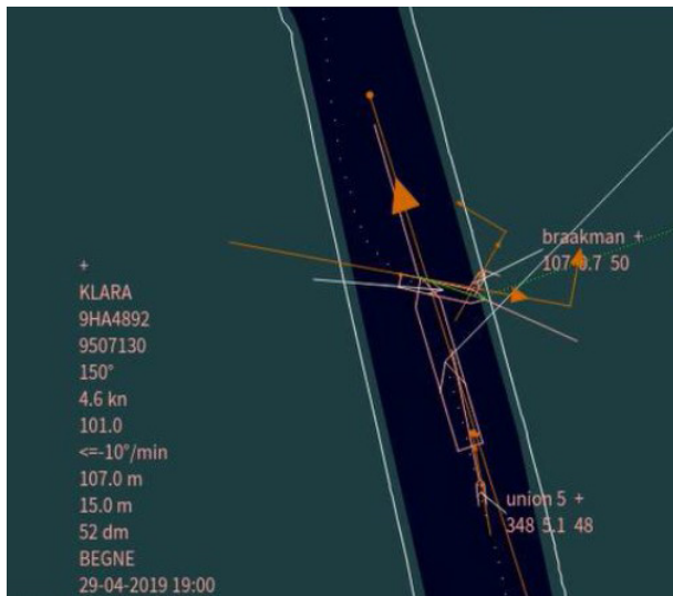
VTS image shortly before M.V. Klara takes the sheer to port. Source – page 5 of MSIU report 09/2020
